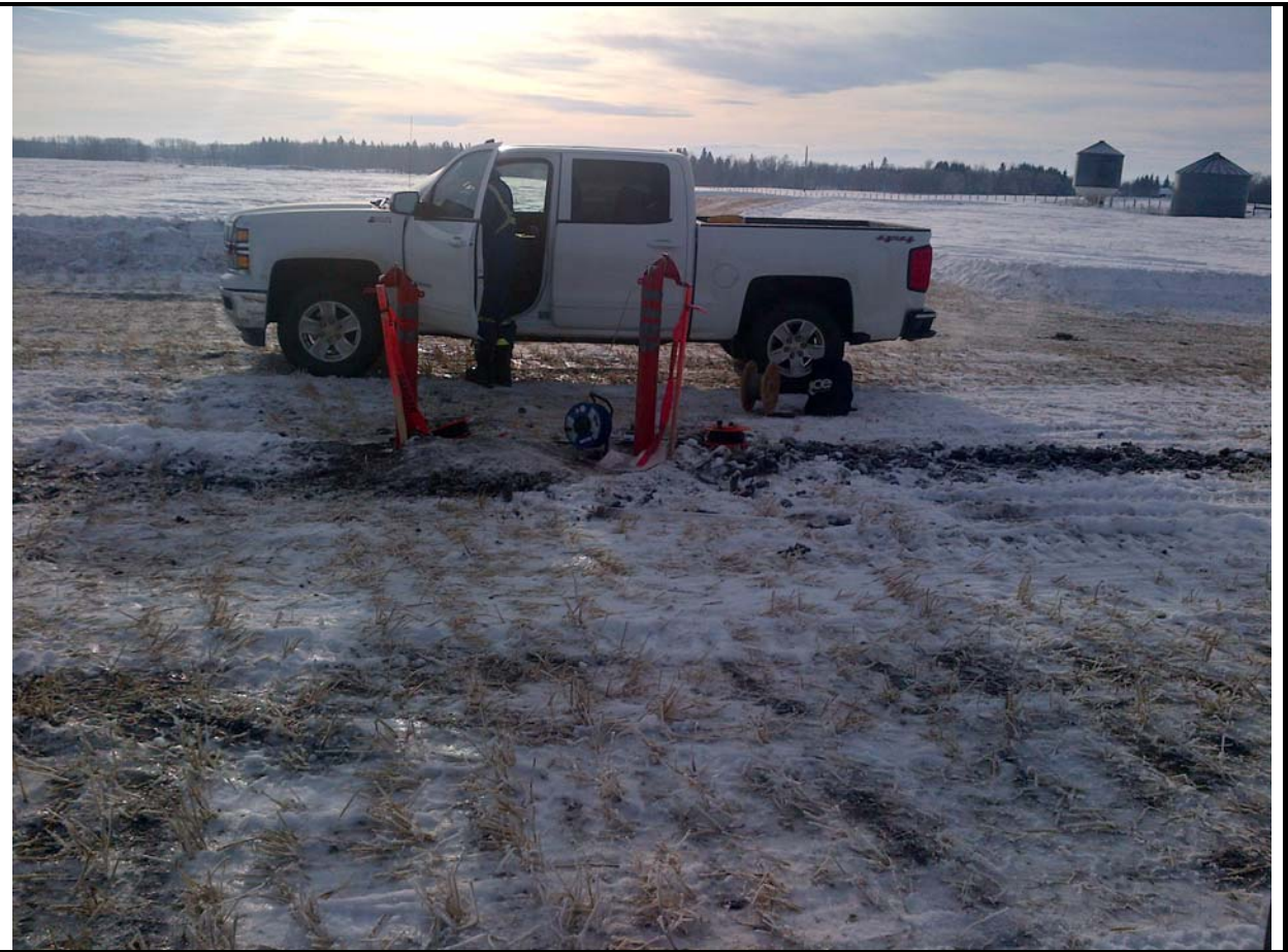
Nested monitoring wells at MW14-5
