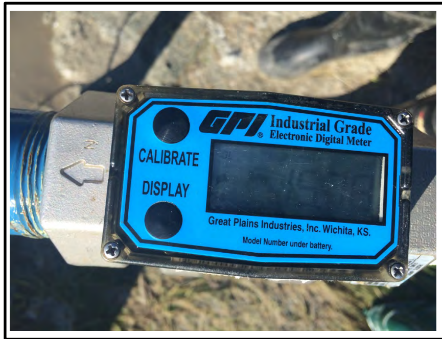
Flow rate meter used in all pumping test measures USgpm
