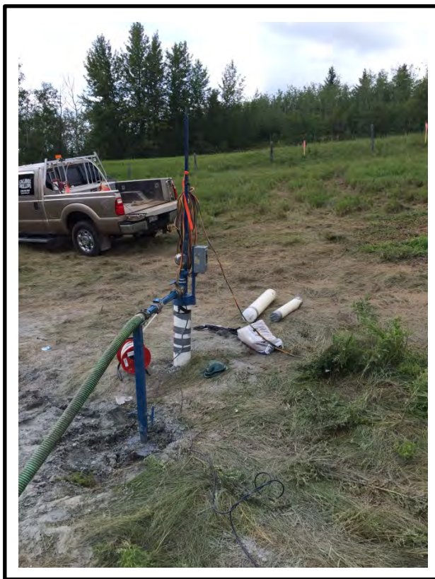
Set up for Step Test/Pumping Test at SE-1
