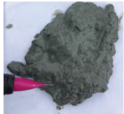
Sand from interval where screen was installed The pencil lead is 0.7mm
