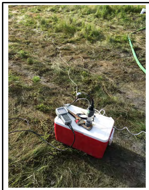
YSI set up during pumping Test
